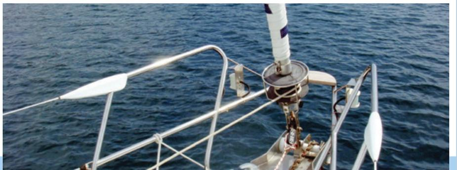
**Universal CROSS-TREE Cover** is the first and unique flexible cross-tree cover to fit all cross trees from 100 mm to 360 mm circumference. It provides ideal protection for all sails. Flexible Integral Skin Foam technology. Easy to fit with a 3m length polyester line included.
