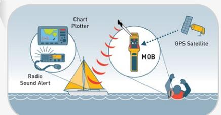
The MOB1 is intended to be installed within the life-jacket and will activate automatically on inflation, sending the first alert within 15 seconds. The MOB1 is waterproof to 10 metres.
